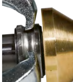
Lock on ball grooves and bearing races.
