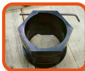
TWLC15 split adapter, closed position
