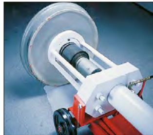
The photo above shows the Universal Puller in position on the roller bearing assembly, which is ready for removal.
